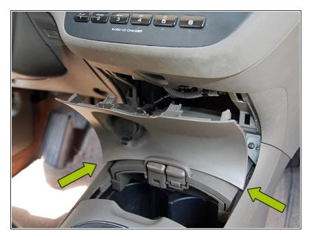
First start by removing the plastic cover under the radio by pulling at the bottom corners.
