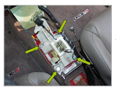
Using 12mm socket and ratchet, remove the (4) M8 mounting bolts on the base of the shifter and
