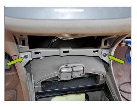
Using a Phillips head screwdriver remove the (2) screws closest to the front of the car.
