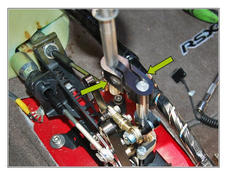
Slide the offset with the upper shifter arm attached, onto the lower shifter arm on the shifter. Adjusted where desired and tighten in place with a 5mm allen key.
