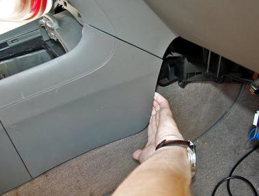
• Reach behind the front lower side on each side of the center console and pull gently to unsnap it
