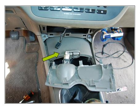
Unplug the connector from the aux power port and remove the cover.
