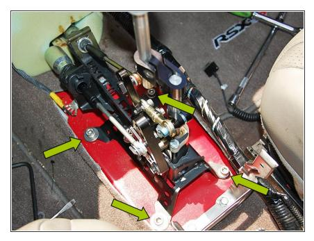
Using the (4) M8 bolts, (4) flat washers, and a 6mm allen key, mount the shifter to the center tunnel.
