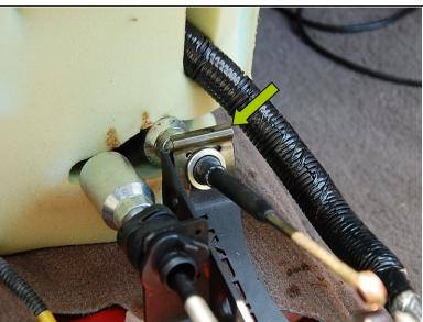
Next slide the right side cable into the shifter (1st picture) and install the C-clip to secure the cable (2nd picture).
