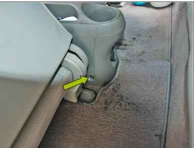
Slide both front seats forward to reveal the final (2) screws holding the center console in. Using the same Phillips head screw driver remove each screw.
