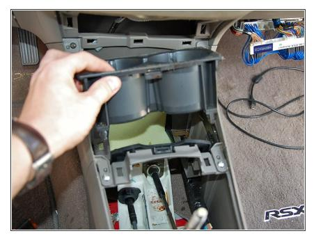
Slide the center console slider forward and remove the cup holder.
