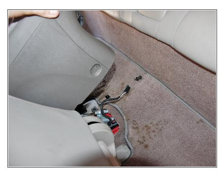
Lift up on the back side of the center console and unplug the rear aux power connector.
