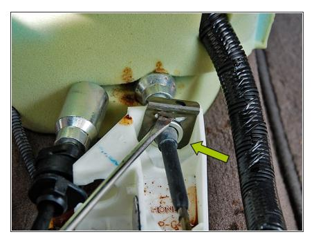
Again using the same flat head screwdriver, pry off the C-clip and slide the cable up out of the shifter.
