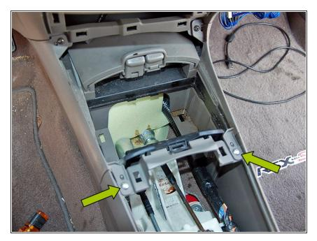
Using the same Phillips head screw driver remove the next set of screws just below the first ones in front of the shifter.
