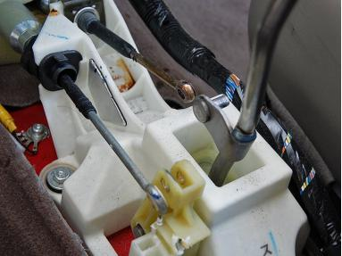
Use a small flat head screwdriver and bend the cotter pins straight, remove both cotter pins securing the cable end links to the shifter and pull them off the shifter.
