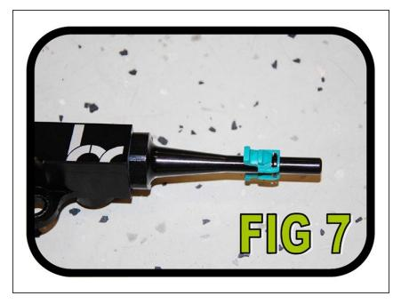
Remove the blue quick disconnect clip from the OEM fuel rail and slide it onto the -8 to 5/16 quick disconnect union as illustrated in FIG 7.
