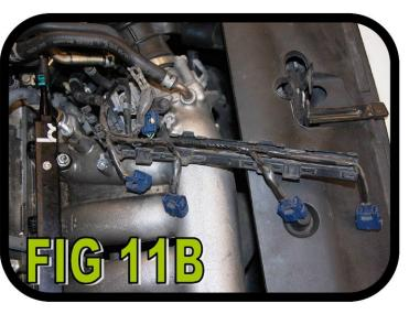
Next we need to remove the plastic cover on the injector wiring harness so we can relocate it.
