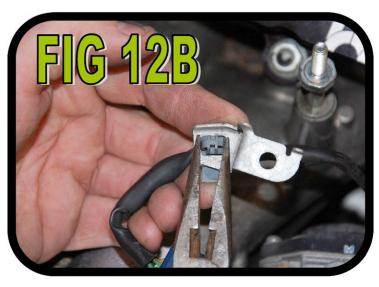
Using a 10 mm socket, remove the metal plate the MAP sensor wire is clipped to. Then, with some pliers, squeeze the clip and pull the wire off of the metal plate. (FIG 12A and FIG 12B).
