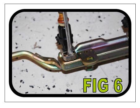
Using a flat-head screwdriver, pull the clips off holding all four (4) injectors in the stock fuel rail as shown in FIG 6. Note: Once you pull one injector out, fuel is going to flow out of the fuel rail. Make sure you have something ready to catch it.
