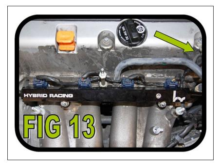
• Plug all four (4) injectors back in. Then, using a 10 mm socket, remove the cap nut on the valve cover. Relocate the injector ground wire to that stud and tighten the cap nut back on top as shown in FIG 13. Note: if the correct wire is not on the corresponding injector the car will not run correctly.
