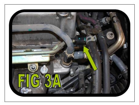
Remove the cap covering the fuel line connection as shown in FIG 3A.
