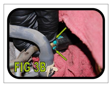
Place a rag around the fuel line, then squeeze the (2) green tabs and pull the fuel line off as shown in FIG 3B. Be careful when doing so as there will likely be pressure in the fuel line.
