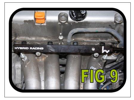
Line the injectors up with the holes on the intake manifold and press the rail onto the intake manifold. Using a 12 mm socket, install and tighten the two (2) nuts holding the fuel rail on (FIG 9).
