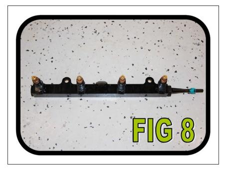
• Install the four (4) injectors into your Hybrid Racing fuel rail. Once this is done it should appear as the one in FIG 8. Note: Spread some oil on the O-ring with your finger before installing the injectors to help them slide in without getting cut.
