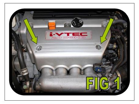
Using a 10 mm socket, remove the two (2) caps nuts holding the cover in place (FIG 1). Once these are removed, pull the cover off. This will take some force. The cover is held on with rubber grommets.
