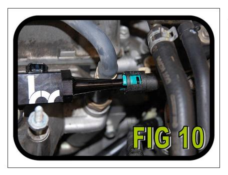
Reconnect the fuel line on the quick disconnect fitting. Do not re-install the cover that you removed in step 3A. (FIG 10)
