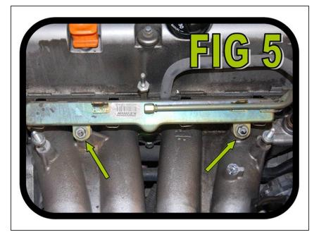
Using a 12mm socket, remove the two (2) nuts holding the fuel rail on and pull the fuel rail off the intake manifold as illustrated in FIG 5.
