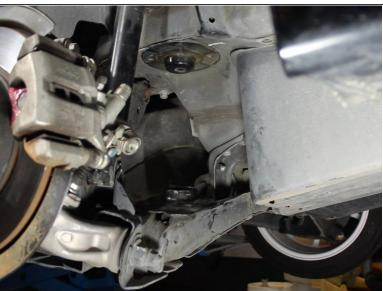
Press down on the brake rotor to push down the lower control arm. This will depress the spring and allow it to be removed.
