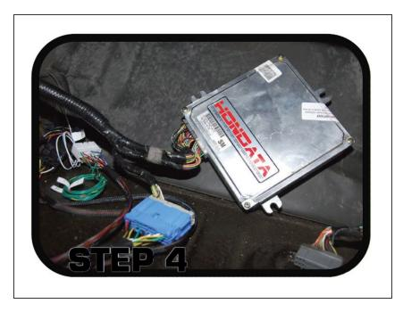
• Grab your ECU and HR conversion harness and move inside the car. Pull back the carpet, kick panel, and remove the stock ECU. You should now have your K-series engine harness, the STOCK K-series ECU, STOCK OEM ECU connectors and the HR conversion harness ready to go.
