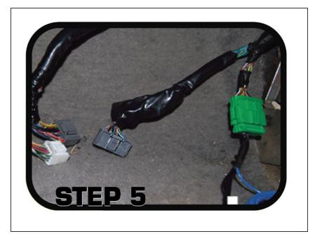
Locate the factory A plug that remains in the car under the dash on the passenger side. This should be a grey connector with 32 pins and is located next to a GREEN CONNECTOR.
