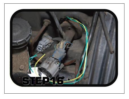
• Route the three (3) loose wires through the grommet located on the driver side firewall. Once the wires are in the engine bay, follow the instructions on the remaining pages to connect them (NOTE: You can also pull the large engine harness connector inside the cabin to clean things up.)
