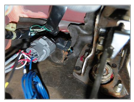
Connect the C101 connector to the HR harness and cut the zip tie on the bundle of wires. Go ahead and secure the connectors with zip ties and move to the next step.
