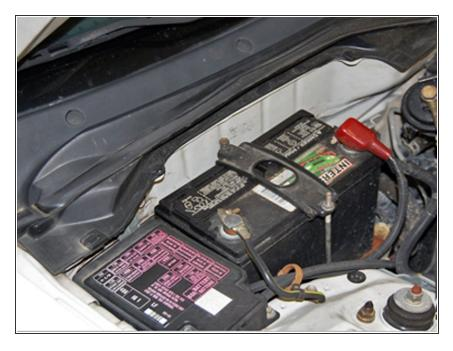
Remove the battery, and battery tray. Once all of these things are out of the way you should be staring at a Grommet on your firewall held in with two (2) 10 mm bolts. This is where your OEM engine harness entered the cabin.
