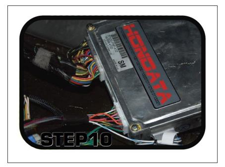
Plug the K-series engine harness into the K-series ECU. Plug the white E plug connector from the Hybrid Racing harness into the ECU.
