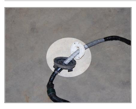
Remove the OEM grommet from your K-series engine harness as well as from your stock D/B series engine harness. You are going to use the one from your old engine on the new K-series harness.
