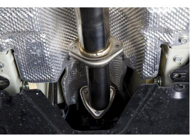
With both gaskets installed on the front pipe adapter, install it on the car. Be sure to keep the bolts loose for the time being.
