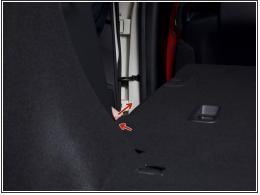
Route the power harness around the corner of the rear seat and down through the rear panel.
