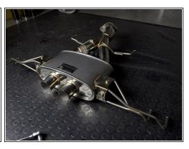
• Locate and install the rear muffler brackets with the supplied hardware. Thread both sides together and be sure to keep them loose so the system can be adjusted once on the car.
