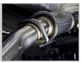
• Use the supplied hardware and attach the pipes together. Finger tighten the bolts right now.
