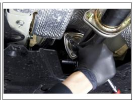
Tighten the exhaust system, starting at the forward most part.
