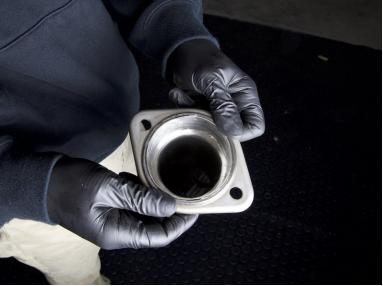
On the other end of the connection pipe, install the correct ring gasket.
