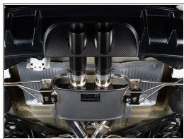
Once the hangers and pipes are tight, tighten the exhaust tips in alignment of the panel.
