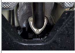
Use the supplied hardware and install the front pipe adapter.
