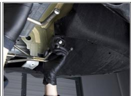
Using the OEM hangers, install the rear HR exhaust section.
