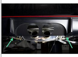
Install the HR carbon rear panel into the bumper using the factory clips. This panel should sit flush at the top and around the bumper seam.
