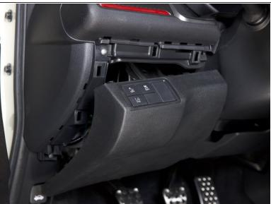
Pull outward on the bottom section of the lower dash panel. It should pop outward allowing you
