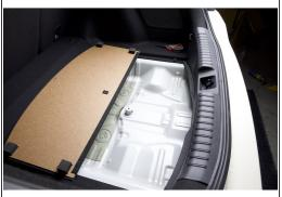
Begin installing the electronic valve controller by lifting and removing the factory FK8 rear foam tray.
