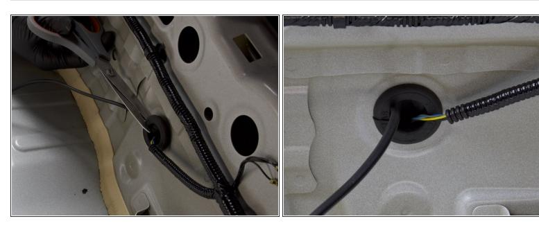
• Use a pair of scissors or knife and cut a slit into the factory grommet. Feed the wire through the slit and re-install the grommet in place.
