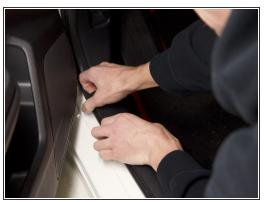
Route the harness under the panels along the sill. You can tuck the wiring under the panels, under the seat belt mount.
