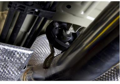
Begin by installing the mid-section of the HR exhaust. You can take this section and hang it from the center hanger.
