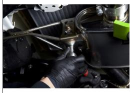
Once everything is aligned, tighten the rear muffler hangers and the remaining pipe connections.
