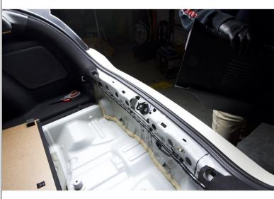
Pull upward on the rear plastic panel to remove it. Once removed, set aside.
