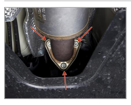
Remove the exhaust from the front pipe.
