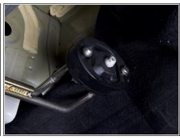
We suggest just installing one hanger through the bushings at a time. Once you have one hanger in each bushing, you can rotate the rubber and get the other one through.
