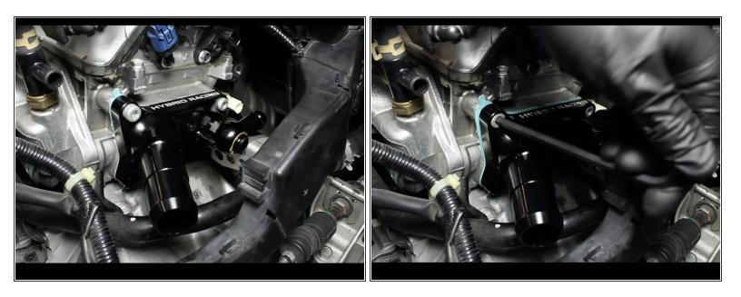
Install the new coolant port housing and tighten them in a crossing sequence.
