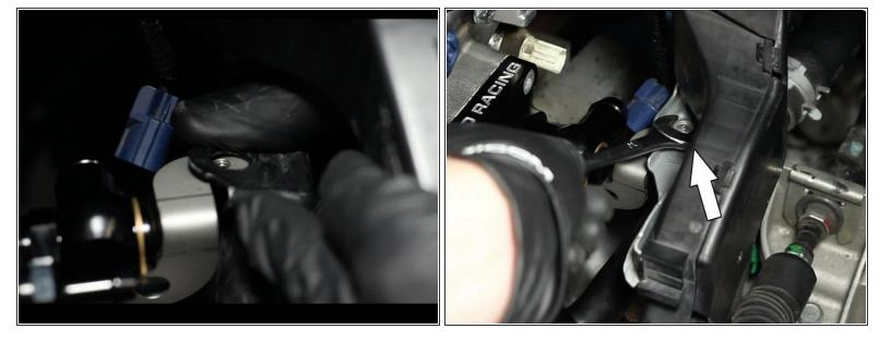
• Bend the heat hose pipe mounting tab back into place and install the factory mounting bracket.
