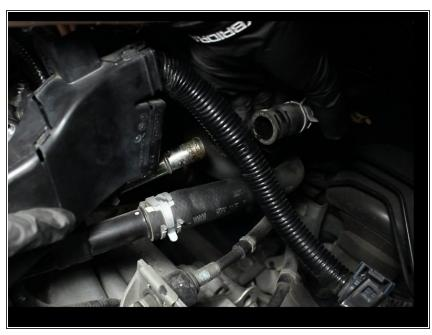
On the rear of the coolant housing, remove the heater hose.
