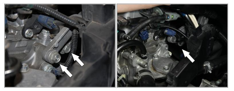
Remove the OEM air intake support bracket.
