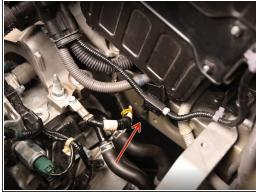
Install the provided clutch line mounting clips.
