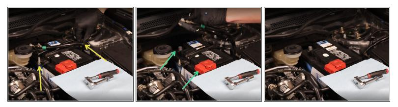
Begin by disconnecting the battery and removing the battery tie-down bracket.
