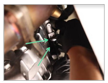
Remove the clutch line at the slave cylinder.
