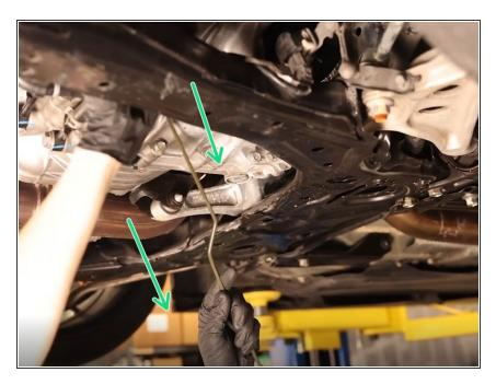
Remove the clutch line from the car.
