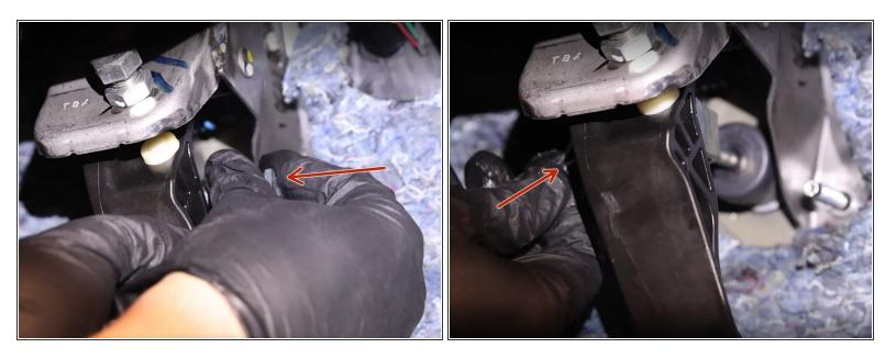
Install the greased clevis and then reinstall the OEM retaining clip.
