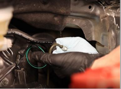
Use a hardline wrench and unbolt the clutch line from the CMC.
