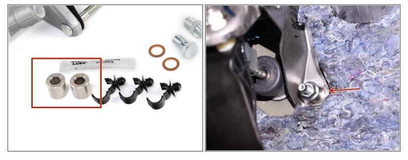
Install the mounting spacers and secure the CMC with the factory 12mm nuts.
