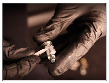
i Use the tube of supplied grease and apply it to the clevis pin.
