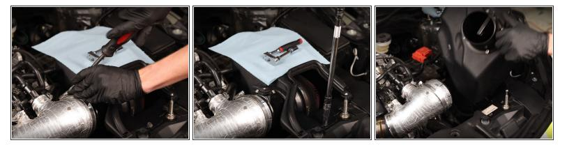
Unbolt and remove the airbox up to the inlet pipe. This will help you access the lower section of the slave cylinder.
