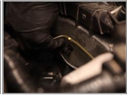
Unclip the clutch line and remove it from the car.
