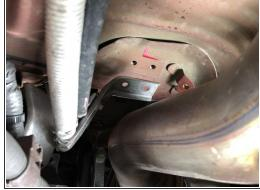
Once the heat shield is out of the way, located the 10mm nuts and bolts holding the shifter cables in place.
