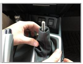
Begin by pushing the shift boot collar down and use a wrench to loosen your shift knob.
