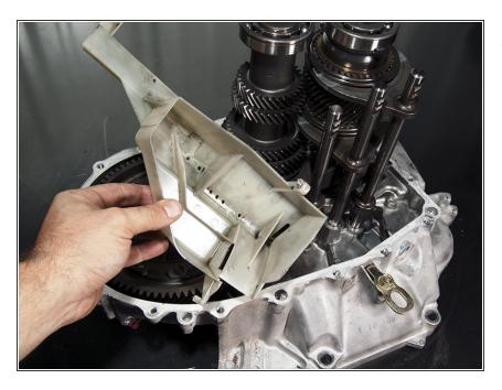
Remove the oil gutter plate.
