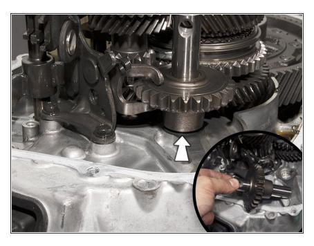
Remove the reverse gear idler and reverse gear shaft.
