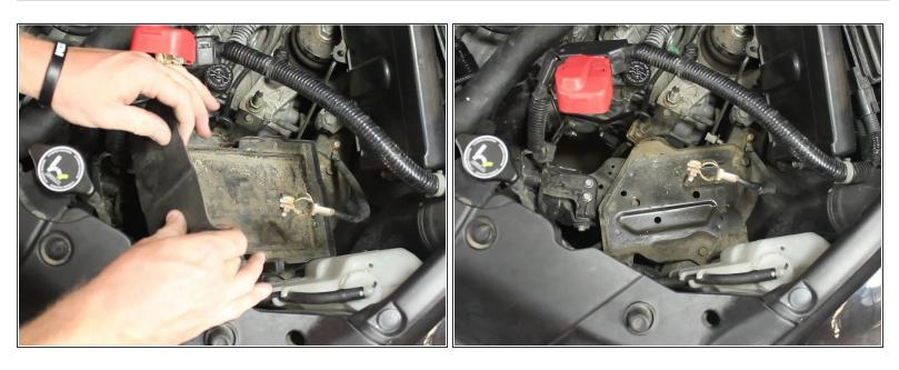
Remove the battery tray cover to expose the battery tray.
