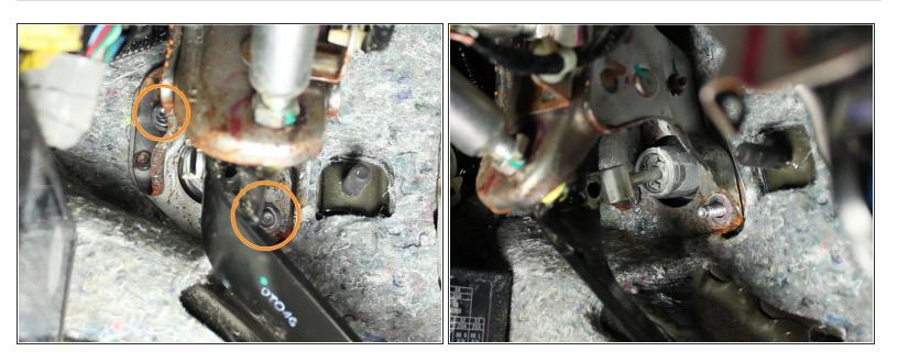
Using a 12mm socket, remove the two mounting nuts that hold the clutch master cylinder in place.
