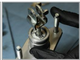
Using the C-clip pliers, insert the OEM rod & fork into the EM1 CMC. The EM1 dust boot is optional.
