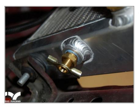
Install the drain bolt. Thread sealer can be used if desired.
