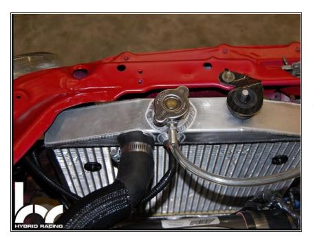
Connect the proper radiator hoses, and fill system with coolant. (radiator hoses may vary due to different
