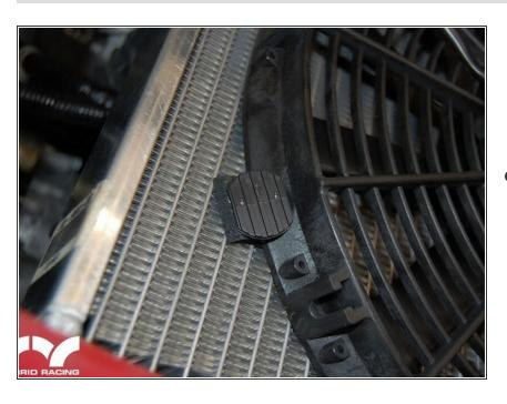
Mount the fan in the appropriate direction and push the tabs through the radiator fins. Install the protective squares between the radiator and the fan, making sure not to damage any of the cooling fins.
