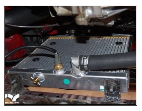
Install the Fan Switch sensor into the bottom bung. (connect to your conversion harness)
