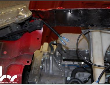
Locate the factory fan connector located near the stock OE radiator fan was. The easiest way to connect the fan is to use the crimp on connectors, remove the stock plug and crimp on the wire connector ends.
