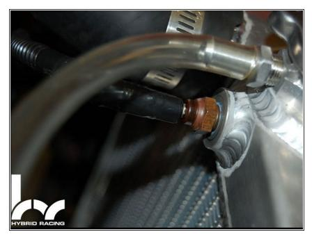
Connect the coolant temperature sensor in the bung at the top of the radiator. (connect to your conversion harness)
