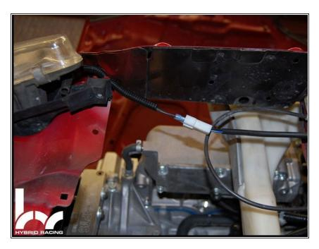
Connect the wires to the new slim fan.
