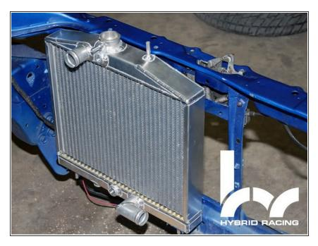
Place the radiator along with the OE rubber grommets into the factory AC location. NOTE: The fan should be attached at this point.
