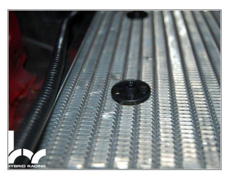
After the tab has been pushed through, clip and slide the back piece and make sure the fan is secured tightly to the radiator.
