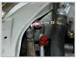
Once the condenser is mounted, install line D which goes from the top of the condenser to the compressor.
