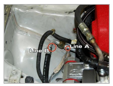
Install the line labeled B. It connects to Line A. Make sure you have an O-ring on the end of line A. The other end will connect to the compressor.
