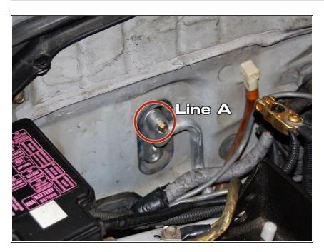
Install line labeled A, starting at the firewall end. Make sure you have the correct O-ring size.
