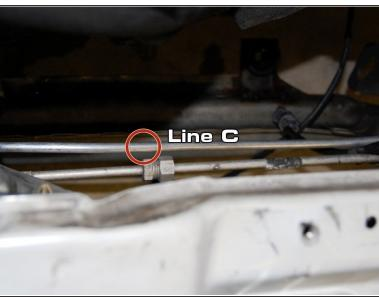
Now it's time for line C. This line comes from the bottom of the compressor to the evaporator. Bolt it to the bottom of the condenser. Make sure not to damage the O-ring, and run the line all the way to the evaporator and install with a 10 mm bolt. It runs alongside the OEM line.
