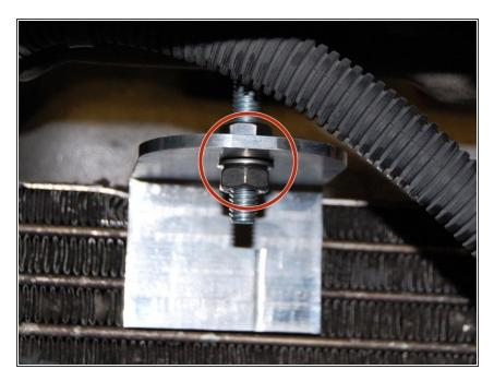
You can now install the EK condenser. Using the supplied brackets and hardware, secure it to the top. If you remove the lower tabs, use the replacements supplied with this kit.
