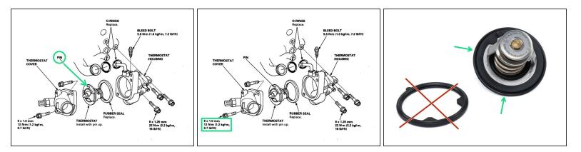
Install with the pin up. Do not install upside down.
