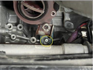
Remove the two 14mm bolts that attach the exhaust manifold to the engine block and remove the support bracket.
