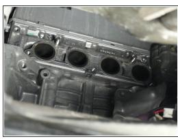
Remove the factory exhaust manifold from the engine.
