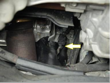
Unplug the primary o2 sensor from the plug that is attached to the firewall by pressing on the release clip.
