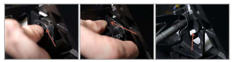
• Rotate the left side shifter cable counter-clockwise and slide it upwards, removing it from the shifter base.
