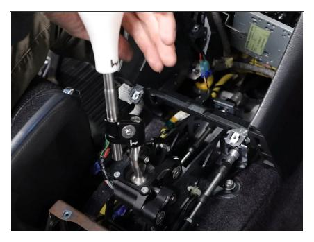
Once the clips are in place, the cables are fully installed. You may now row through each gear. Make sure everything feels good before reassembling your car.
