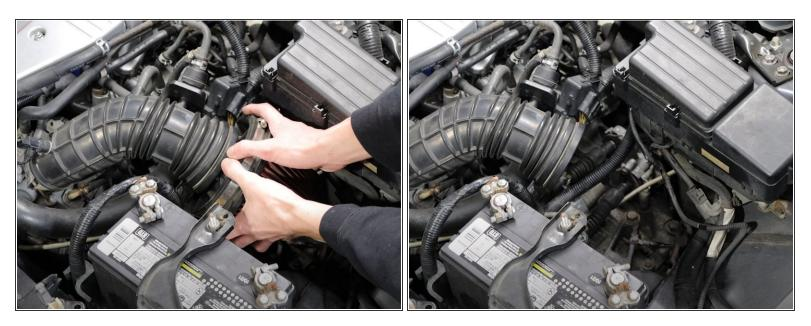
• Remove the air filter, or airbox to gain access to the top of the transmission.
