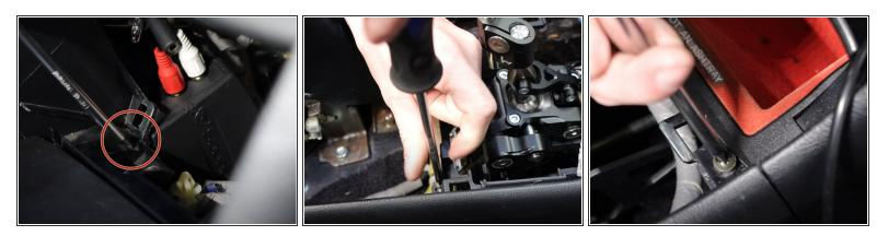
• Remove all of the Phillips screws holding the console and coin pocket in place.
