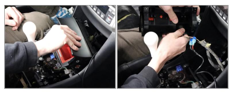
• Remove the coin pocket and unplug the 12v socket.
