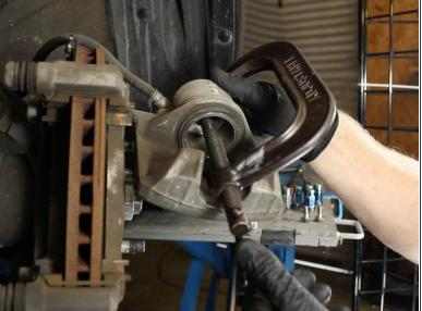
• Using a C-clamp or brake caliper tool to slowly compress the piston. This will allow the housing to be assembled with the new pads.
