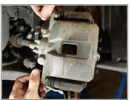
Remove the two 12mm bolts that mount the piston housing to the brake pad housing. This will allow you to separate the two sections for easy access to the pads.
