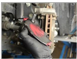
Apply a small amount brake pad lubricant to the back of each brake pad and to each end where the pad makes contact to the caliper.
