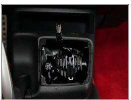
Gently pry the shift boot console upwards. Remove it completely.
