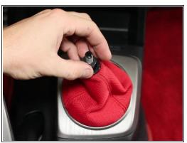
Begin by removing the shift knob & locking nut. (if equipped)
