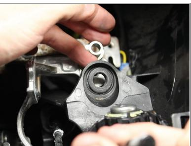
Push the metal base out of the rubber bushing.
