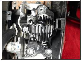
Once the shifter assembly has been fully exposed, remove the 3 mounting bolts.
