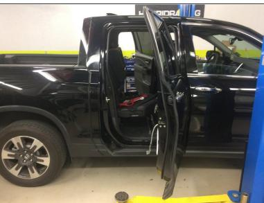
Using the OEM front stops on the rear door allows the rear door to open further. This creates more room for loading long objects into the rear of the cab.
