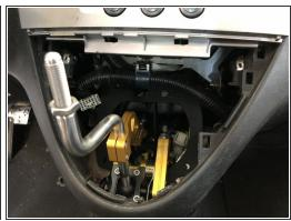
Insert your new Hybrid Racing shifter into the dash by holding the dash center out of the way. This shifter is much smaller so it should slide in easy.
