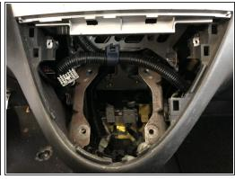
Remove the shifter assembly by pulling the center dash section outwards and upwards. Hold it out
