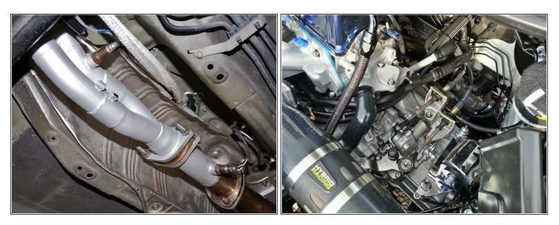
• Finally, using your 10mm socket re-install the heat shield with the (4) M6 bolts and (2) nuts and your installation is complete!
