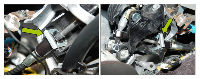
Push the bushings into the correct place on the back side of the shifter and slide on the "c"-shaped linkage clips provided just as you did with the transmission side. When completed yours should look like the ones illustrated in Fig 1/2.
